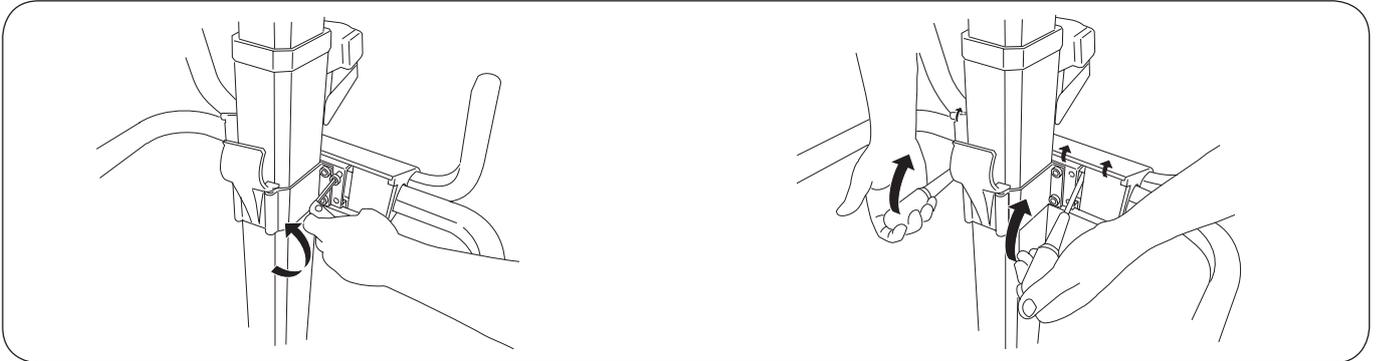
A. Loosen both of the M8 screws on each side of the mast.
